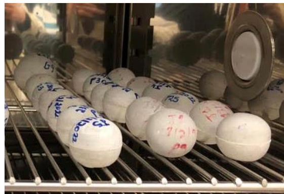
Figure 1: Mortar spheres of 40 mm diameter (model materials)
