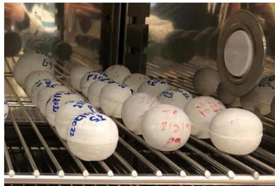
**Figure 1: Mortar spheres of 40 mm diameter (model materials)**
