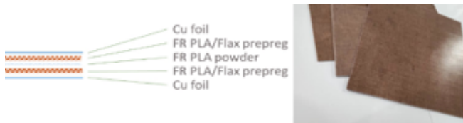
Fig. 2. PLA/Flax laminated substrate [5].
