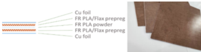
Fig. 2. PLA/Flax laminated substrate [5].
