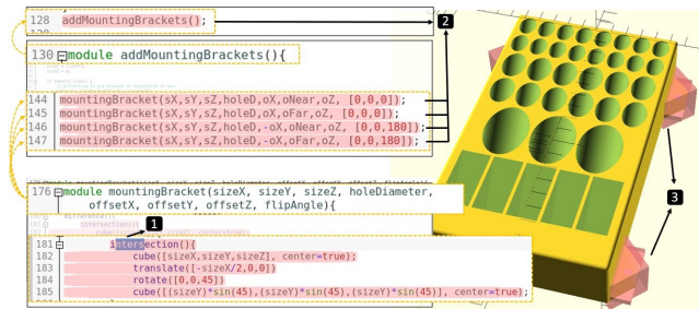
Figure 4: Forward navigation. F4: After selecting a portion of an instantiating statement, (1) all the instance creations of the selected code are highlighted in pink, and (2) all the resulting elements are highlighted in pink in the 3D view (3).
