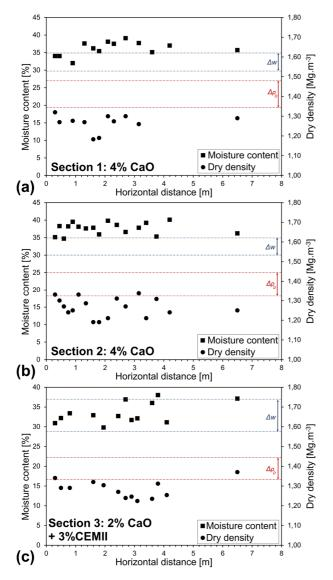
Figure 2. Moisture content and dry density evolution along the horizontal cores for section 1 treated with 4% lime (a), section 2 treated with 4% lime (b), and section 3 treated with 2% lime and 3% cement (c).
