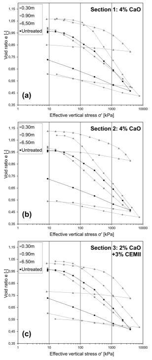
Figure 3. Compression curves of specimens taken from various horizontal distances for section 1 treated with 4% lime (a), section 2 treated with 4% lime (b), and section 3 treated with 2% lime and 3% cement (c).
