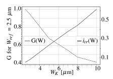
Fig. 5. Variation of the threshold current  $i_{tr}$  in black line and post-threshold activation function gain G with the width of  $MN_K$
