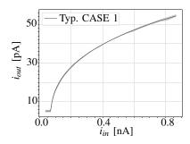
Fig. 6. Activation function of the  $eN_1$ . Changing the width  $W_{DEN,1}$  of the next-layer dendrite cause the AF to slightly deform, as it's plotted by the blue surface (functions  $AF((W),i_{in})$ ). Relative standard deviation is  $\sigma = 1.8$ % and the maximum deviation is 0.8 pA
