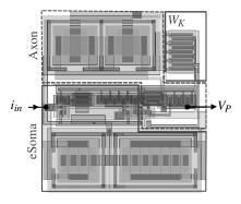
Fig. 3. Layout of an eN without dendrites in the maximum area configuration for  $W_K=10~\mu m$  (on the top right corner). Area is  $10.8\times 9.7~\mu m^2$ .
