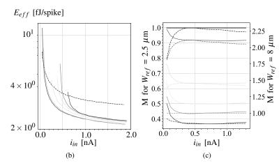
Fig. 4. (a) Activation function for 8 values of  $W_K$ . Reference activation function has  $W_K = 2.5 \mu m$  (b) energy efficiency against the input current  $i_{in}$  of the eN. (c) present the variable  $M(i_{in})$ , representing the post-threshold gain. In continuous line, M is computed for  $W_{ref} = 8 \mu m$  and  $2.5 \mu m$  for the dashed one.
