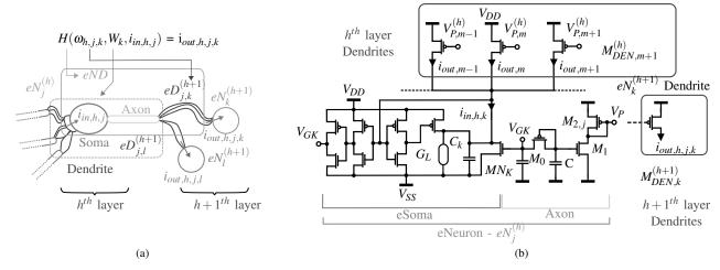
Fig. 1. (a) Biological inspired neural network topology. Each soma is connected to one axon and make connections through dendrites. (b) Schematic for an analog neuron and dendrites ( $V_{DD} = 100 \ mV$ ,  $V_{SS} = -100 \ mV$ ). For each new connection, a single PMOS transistor (dendrite) is added to form a new synapse. Transistor sizing is obtained from [11]. Modified sizing are:  $M_0$  with 810/60 nm;  $M_{2,i}$  with 2100/60, C = 16.88 fF,  $M_1$  with 135/60 nm.
