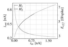
Fig. 2. Energy efficiency and *eND* behavior for two driving methods. Blue represent those functions for a *eND* driving circuit and green in a case of a constantly biased PMOS driving circuit.
