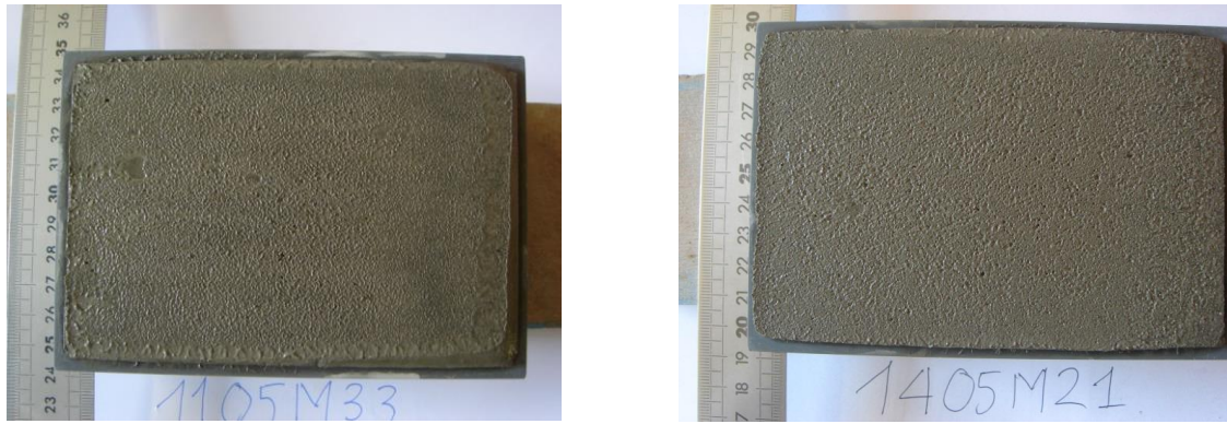
Fig. 5 Textures of the tested mortar samples at 5V,10V, 20V, 30V at 11^\circ (left) and 14^\circ (right)
