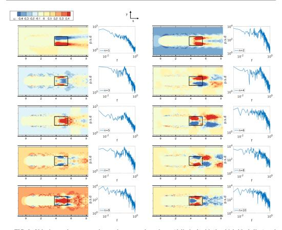
FIG. 8. Velocity modes computed over the near-wake volume (delimited with the thick black line) and extended to the full domain, viewed in a horizontal plane at midheight.
