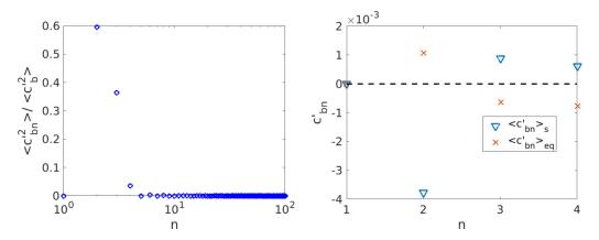
FIG. 6. (Left) Relative contribution of the POD modes to the variations of the base pressure coefficient (see text). (Right) Contribution of the modes corresponding to the characteristic states  $a_n^{p,eq}$  and  $a_n^{p,s}$ .
