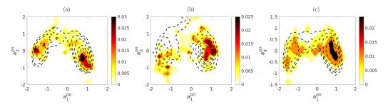
FIG. 4. Comparison of the joint histograms of the POD amplitudes  $a_1^{pn}$  and  $a_k^{pn}$  for k=2,3,4. The color contours correspond to the numerical data. The dashed line contours correspond to the same levels for the experiment. The contour levels are the following: (a) k=2:0.003,0.005,0.01,0.02,0.03; (b) k=3:0.0025,0.005,0.01,0.024; (c) k=4:0.002,0.005,0.01,0.015,0.02,0.025. A moving average of 10 convective time units was used.
