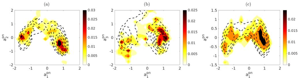
FIG. 4. Comparison of the joint histograms of the POD amplitudes  $a_1^{pn}$  and  $a_k^{pn}$  for  $k = 2, 3, 4$ . The color contours correspond to the numerical data. The dashed line contours correspond to the same levels for the experiment. The contour levels are the following: (a)  $k = 2$ : 0.003, 0.005, 0.01, 0.02, 0.03; (b)  $k = 3$ : 0.0025, 0.005, 0.01, 0.024; (c)  $k = 4$ : 0.002, 0.005, 0.01, 0.015, 0.02, 0.025. A moving average of 10 convective time units was used.
