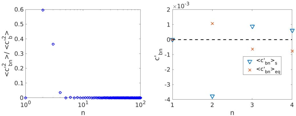
FIG. 6. (Left) Relative contribution of the POD modes to the variations of the base pressure coefficient (see text). (Right) Contribution of the modes corresponding to the characteristic states  $a_n^{p,eq}$  and  $a_n^{p,s}$ .
