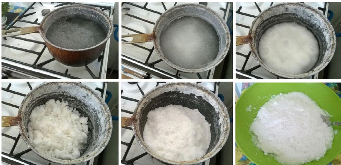
Figure 7. Making fine, white table salt by boiling the brine (experiment by F. A. Tencariu).
