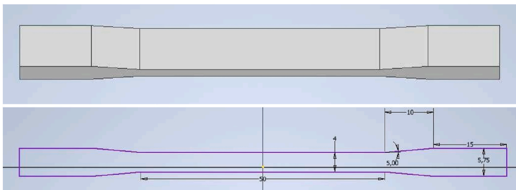
Fig. 1. Shape and dimensions of the test piece (units: mm for dimensions and ^\circ for angles).
