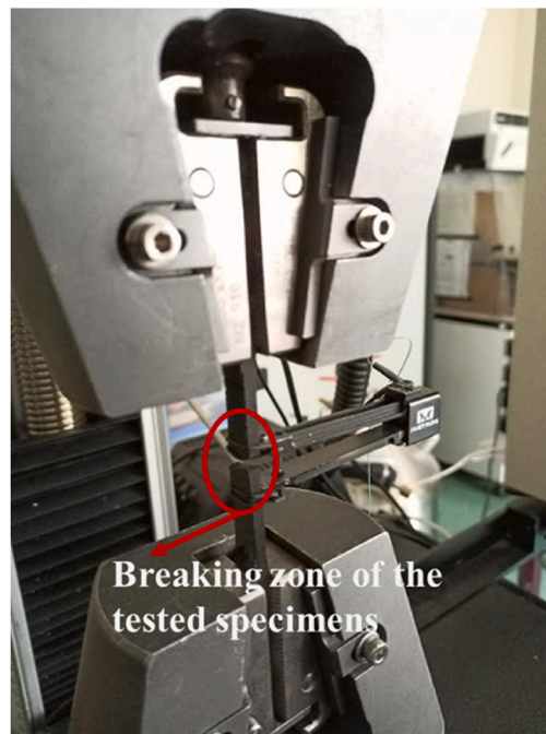
Fig. 5. Tensile test and breaking zone of the specimens.
