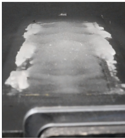
(a) Experimental visualisation of the ice shape for Test 04 at t = 100s
