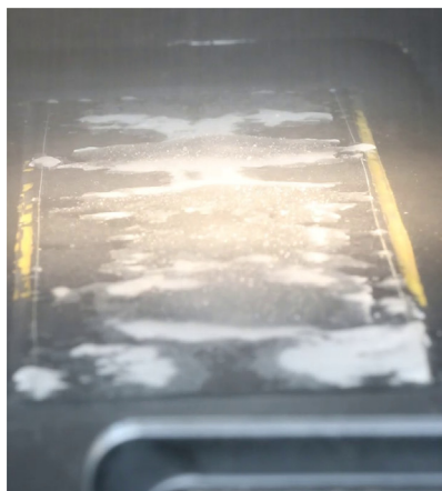
(a) Experimental visualisation of the ice shape for Test 28 at t = 100s
