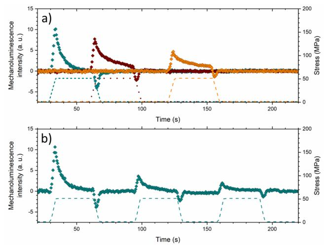
6 S1. Mechanoluminescence of GC-1200 a) with different delay times before applying the load b) under
