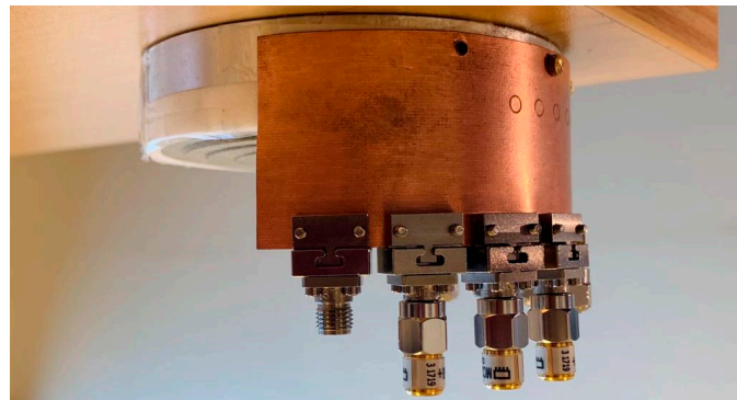
Figure 28. Patch antenna feeding the Luneburg lens.
