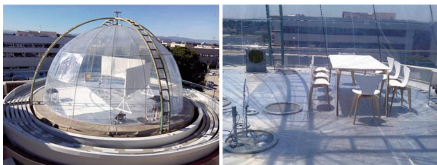
Fig. 7.13 Photocatalytic materials in the EUPHORE chamber. Left: textiles on structures and on the ground. Right: outdoor furniture
