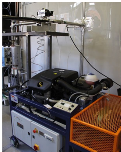
Fig. 5.16 Schematic of engine injection set-up at the University of Manchester
