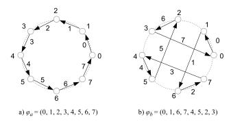
Fig. 3. Permutation of an 8-PSK NB-CCSK sequence
