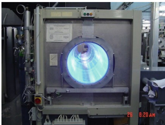
Fig. 1.12 QUAREC chamber, Wuppertal, the lights are mounted outside the chamber providing a uniform radiation field in the actual chamber
