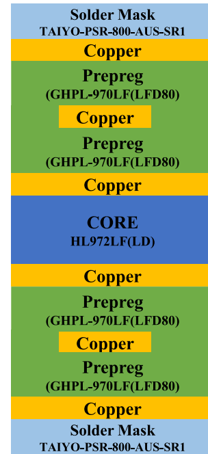
Fig. 6. Schematic cross section of the six metallic layers organic substrate designed and manufactured for flip-chipping the BiCMOS 55-nm die.
