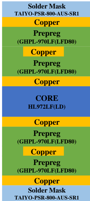
Fig. 6. Schematic cross-section of the 6 metallic layers organic substrate designed and manufactured for flip-chipping the BiCMOS 55 nm die.
