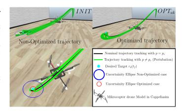
Fig. 1. Drone trajectory tracking under parametric uncertainties (green) to reach a target  $s_d(t_f)$  (light blue sphere). Non-optimized (INIT), top left) and optimized  $(OPT_{ak})$ , top right) trajectories are compared. The size of the uncertainty ellipses are compared in the bottom left, where the blue and red ellipses correspond to INIT and  $OPT_{ak}$ , respectively. A video demonstration is available at: https://youtu.be/VBRL8XDiJ5c.
