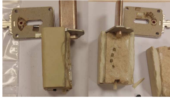
Figure 3 : Cutting of a new (left) and a blown (right) aR fuse.
