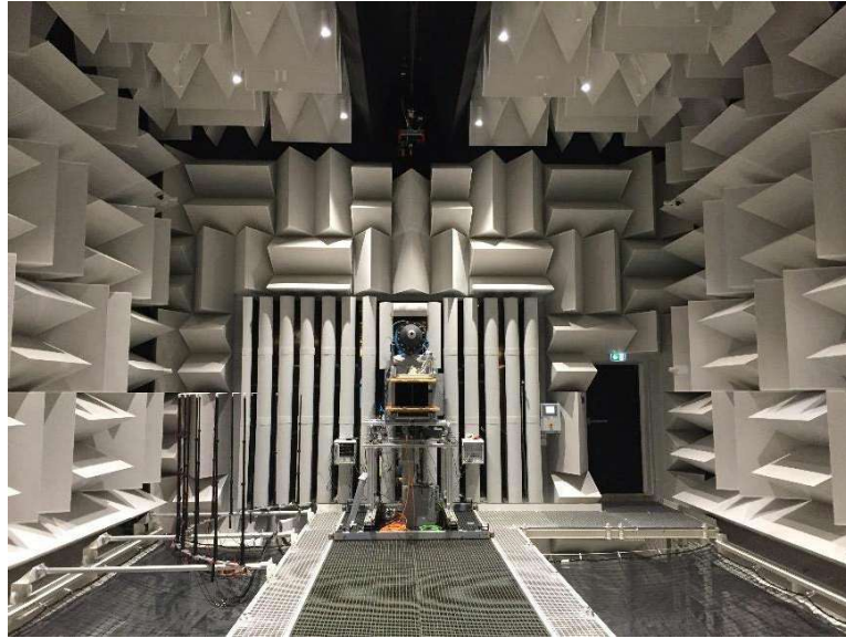
Figure 1. Picture of the subsonic and supersonic anechoic wind tunnel at LMFA.
