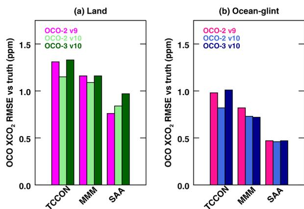
**Figure 1.** RMSEs for different versions of OCO-2 and OCO-3 XCO<sub>2</sub> versus three truth proxies: TCCON, multi-model median (MMM), and small area approximations (SAAs). Results are derived from single-sounding statistics using quality-filtered and bias-corrected XCO<sub>2</sub> from the QTS. Results for land observations are shown in panel (a), while panel (b) shows results for ocean-glint observations.
