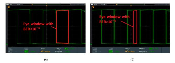
**Figure 11.** Eye diagrams for OOK and BFSK VLC prototypes evaluation: (a) BFSK modulation at  $\approx$ 3500 µW/cm<sup>2</sup>; (b) BFSK modulation at  $\approx$ 3600 µW/cm<sup>2</sup>; (c) OOK modulation at  $\approx$ 2800 µW/cm<sup>2</sup>; (d) OOK modulation at  $\approx$ 2900 µW/cm<sup>2</sup>.
