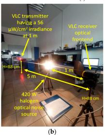
**Figure 9.** VLC prototype optical noise resilience evaluation: (**a**) envisioned testing setup; (**b**) experimental testing setup.
