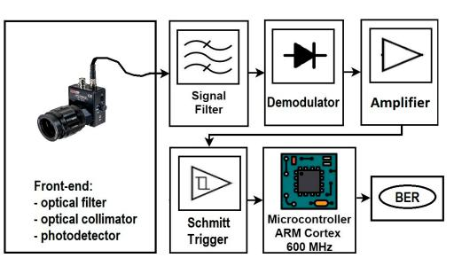
Figure 6. Schematic representation of the VLC BFSK receiver system used in these experiments.
