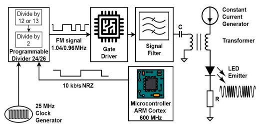
Figure 2. Schematic representation of the VLC BFSK emitter system used in these experiments.
