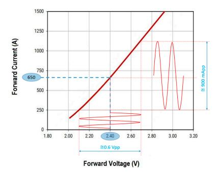
Figure 4. Electrical characteristics curves for XP-E2 LED.
