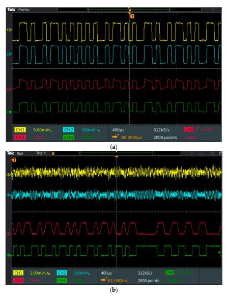
**Figure 10.** Oscilloscope print-screens showing the signal regeneration process at the level of the different stages of the VLC receiver: Channel 1 (yellow) shows the output of the transimpedance amplifier; Channel 2 (blue) shows amplified Channel 1 signal; Channel 3 (purple) shows the adaptive gain control circuit, and the output of the demodulator, respectively; Channel 4 (green) shows the regenerated signal after Schmitt trigger circuit: (a) OOK modulation; (b) BFSK modulation.
