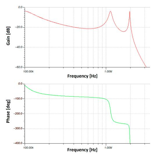
Figure 3. Bode plot for the emitter low-pass filter.
