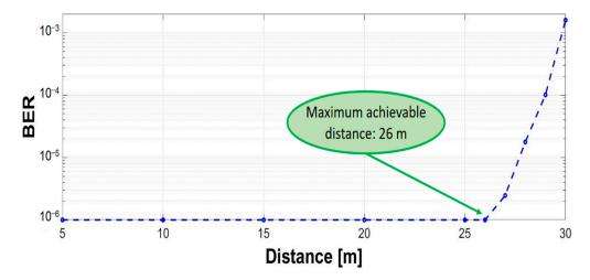
Figure 7. Maximum achievable distance with the VLC BFSK prototype.
