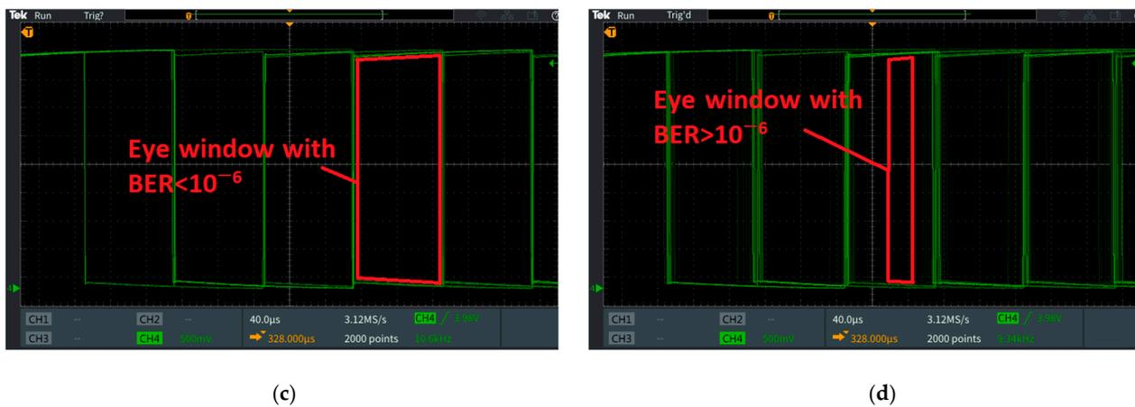
**Figure 11.** Eye diagrams for OOK and BFSK VLC prototypes evaluation: (a) BFSK modulation at  $\approx 3500 \mu\text{W}/\text{cm}^2$ ; (b) BFSK modulation at  $\approx 3600 \mu\text{W}/\text{cm}^2$ ; (c) OOK modulation at  $\approx 2800 \mu\text{W}/\text{cm}^2$ ; (d) OOK modulation at  $\approx 2900 \mu\text{W}/\text{cm}^2$ .
