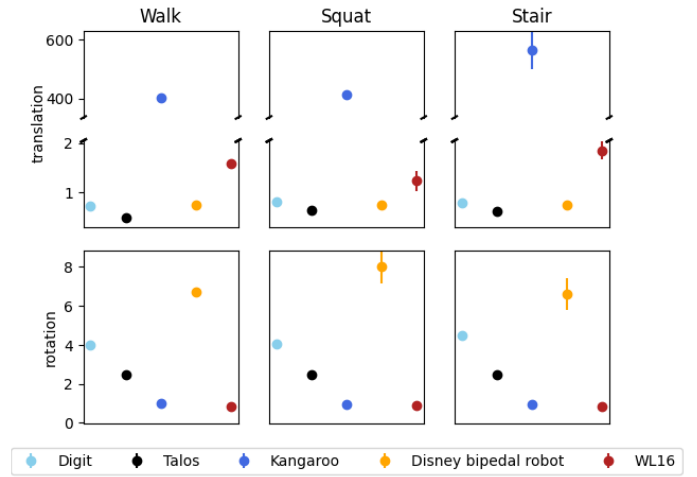
Fig. 4. Velocity manipulability of the foot, in translation (TM, top) and rotation (RM, bottom)
