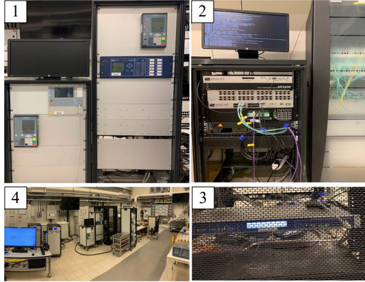
Fig. 3: Laboratory setup. 1: Physical PMUs, 2: Real time simulator, 3: GPS clock and 4: Panoramic view of the laboratory.
