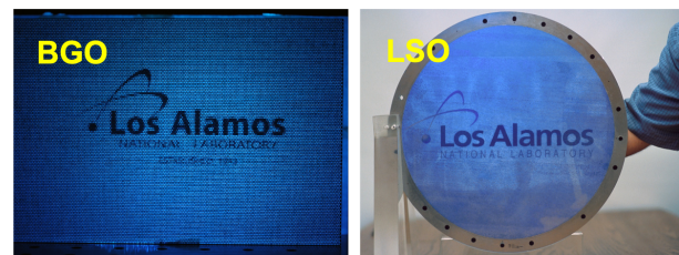
Fig. 9: Segmented BGO and LSO [98] scintillators. Both have 1 \text{ mm} \times 1 \text{ mm} \times 40 \text{ mm} scintillator pixels and are separated by a metal septum.
