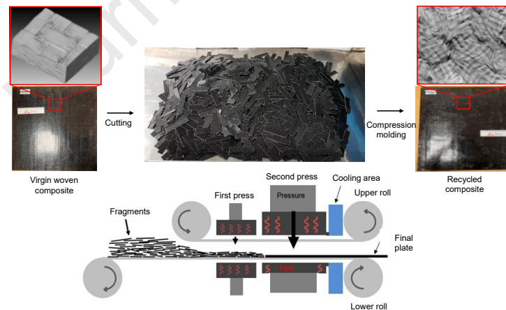
Figure 1: Schematic of the Thermosaic® production line showing the processing steps for mechanical recycling of thermoplastic composites.
