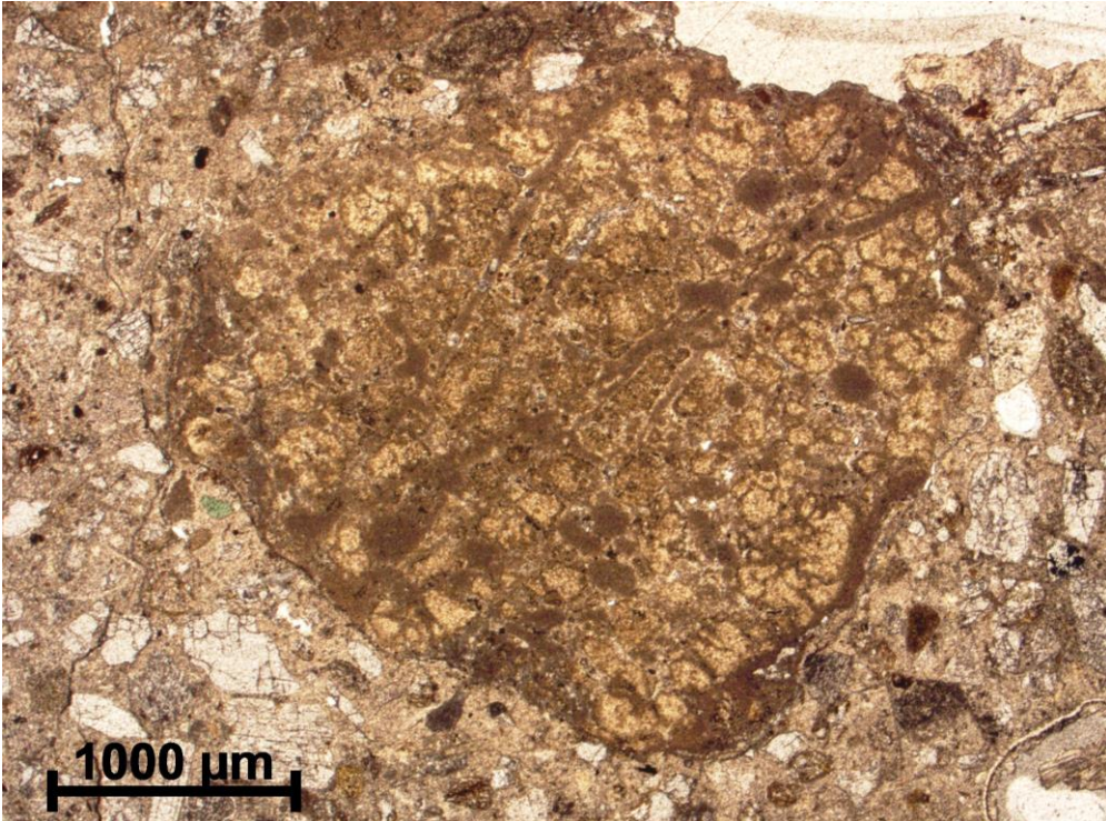
Figure 16 - Thin section in polarized transmitted light. Underburnt fragment of Pietra Alberese indicating that this limestone was the raw material for the production of lime.
