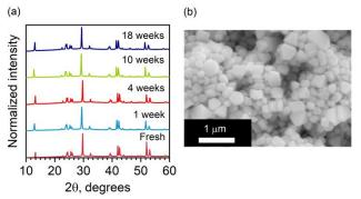
**Fig. 5.** (a) Evolution of the XRD patterns of a AgBil<sub>4</sub> NC film stored in the ambient conditions in dark (RH  $\sim$  40% T = 25 °C). The patterns were recorded under identical measurement settings. (c) SEM image of an aged NC film (two months old) stored in the ambient conditions in dark.
