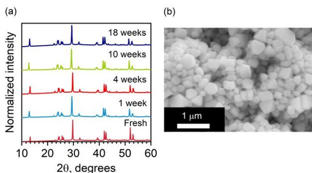
**Fig. 5.** (a) Evolution of the XRD patterns of a  $\text{AgBiI}_4$  NC film stored in the ambient conditions in dark (RH ~ 40% T = 25 °C). The patterns were recorded under identical measurement settings. (c) SEM image of an aged NC film (two months old) stored in the ambient conditions in dark.
