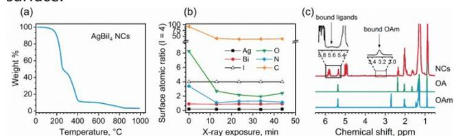
**Fig. 6.** (a) TGA data for a  $\text{AgBiI}_4$  NC sample. (b) Changes in surface composition (atomic ratios normalized to I = 4) of  $\text{AgBiI}_4$  film sample during XPS measurement of five consecutive cycles of spectra (Bi 4f → I 3d → Ag 3d → O 1s → C 1s → N 1s, duration of a cycle ~10 min). (c) <sup>1</sup>H NMR spectra of  $\text{AgBiI}_4$  NCs, pure OA, and pure OIAM. The insets highlight the proton resonances related to bound ligands.
