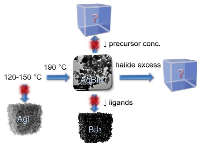
Fig. 1. Schematic representation of the synthesis optimization routes to obtain phase-pure AgBiI<sub>4</sub> NCs.
