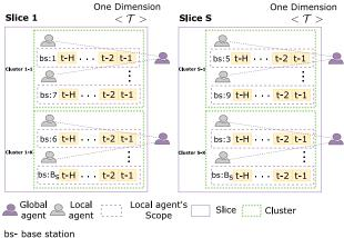
Fig. 4: Problem dimensions of the Clustering-based FPLSTM framework.
