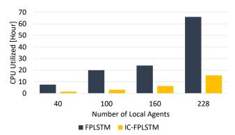
Fig. 15: Per CPU time utilization comparison of FPLSTM and IC-FPLSTM under different number of local agents.
