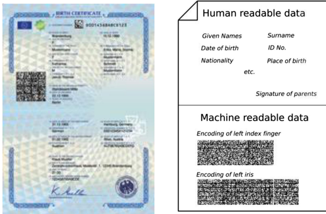
FIGURE 5 Proposed birth certificate from the FIDELITY project [46]. Left: Draft product design. Right: Sizes of barcodes correspond to the approximated storage requirement for the compressed biometric sample.
