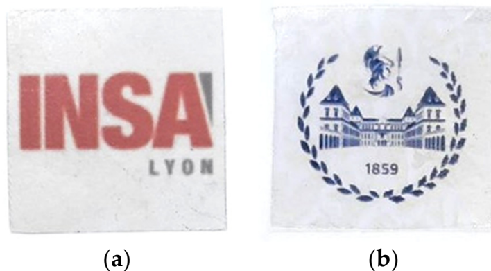
Figure 7. Transparent film of PMMA- co -MAA after compression molding at 230 °C (a) and with the addition of 10 wt% of CNF after compression molding at 230 °C (b).
