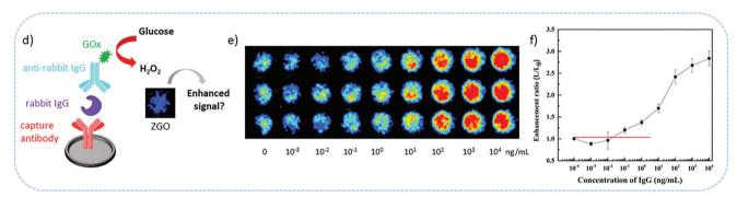
**Figure 5.** a) Principle of antigen detection based on signal enhancement using direct ELISA experiment. b) Persistent luminescence signal versus [IgG]. Experiments done in triplicate (n = 3). c) Signal enhancement versus [IgG]. d) Principle of antigen detection based on signal enhancement using a sandwich ELISA protocol. e) Persistent luminescence signal versus [IgG]. Experiments done in triplicate (n = 3). f) Signal enhancement versus [IgG]. Experiments done in triplicate (n = 3).
