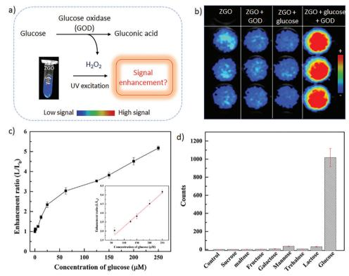
Figure 2. a) Principle of glucose detection based on H<sub>2</sub>O<sub>2</sub> induced signal enhancement. b) Influence of operating conditions on the signal enhancement. c) Linearity area for glucose detection. d) Specificity of the technique for glucose detection. Experiments done in triplicate (n = 3).
