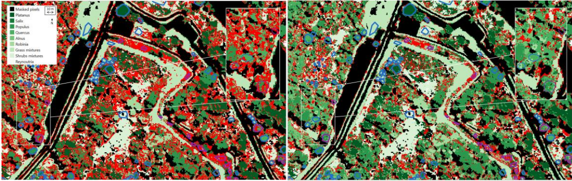
Figure 6. Classification maps of site 2 using RF (left part), SVM-linear (right part) plus rejection with a rejection threshold of 0.2, and in-field data (predominant species are delineated in blue and minor species in purple). Rejected pixels are represented in red.
