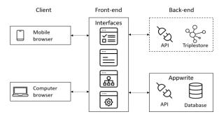
Figure 2. Schema of the architecture of the tool (dashed rectangle not yet implemented)
