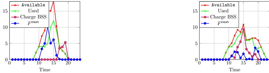
(a) Before storage control: objective is 79.37 kWh, energy injected into MG is 31.10 kWh.
