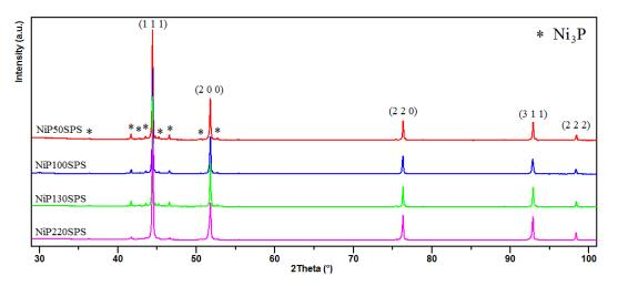
**Figure 2.** XRD patterns of metal matrix composites (MMCs) based on Ni-densified Ni-P samples obtained by reactive spark plasma sintering (SPS) from different particle sizes of nanopowders.
