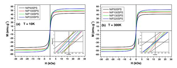
**Figure 7.** Hysteresis loops at 10 (**a**) and 300 K (**b**) of materials produced by reactive SPS (R-SPS) from various particle sizes of Ni-P nanopowders.
