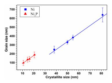
**Figure 4.** Variation of grain size of Ni ( $\blacksquare$ ) and Ni<sub>3</sub>P ( $\blacktriangle$ ) as a function of crystallite size of MMCs.
