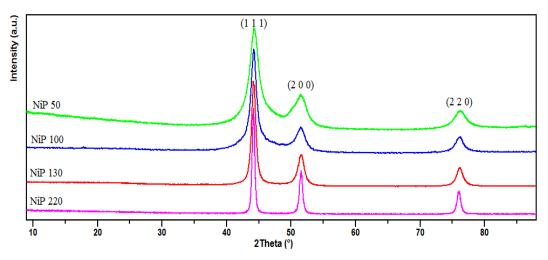
Figure 1. X-ray diffraction (XRD) patterns of starting Ni-P powder.
