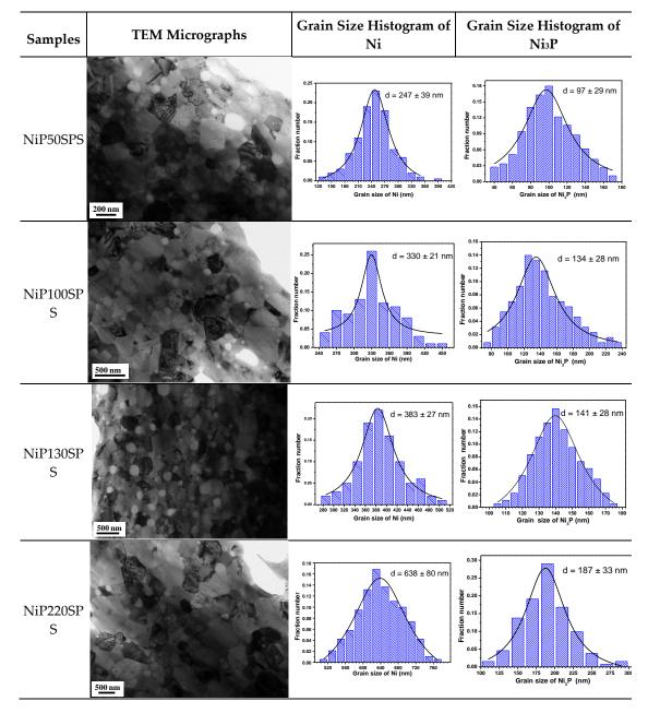
**Figure 3.** Transmission electron microscope (TEM) observations submicrometer grain-sized samples and grain size histogram of Ni and Ni<sub>3</sub>P.
