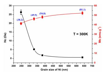
**Figure 9.** Variation of the saturation magnetization (Ms) (●) and coercive field (Hc) (■) at 300 K of the consolidated samples as a function of the grain size of the Ni. At each experimental point, we report, in blue parentheses, the crystallite size of Ni in nanometers.
