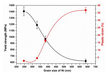
**Figure 8.** Variation of yield stress (**■**) and plastic strain (**●**) for the sintered samples as a function of the grain size of the Ni.
