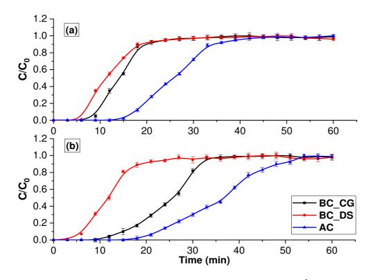
Fig. 4. Thiophene breakthrough curves at T= 500 °C;  $Q_v = 0.1 \text{ Nm}^3/\text{h}$ ; (a) mixture 1; (b)
