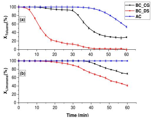
Fig. 5. Synthetic mixture 2,  $ts_2 = 2.50 s$ ; T= 500 °C : (a) Toluene conversion; (b) Limonene conversion.
