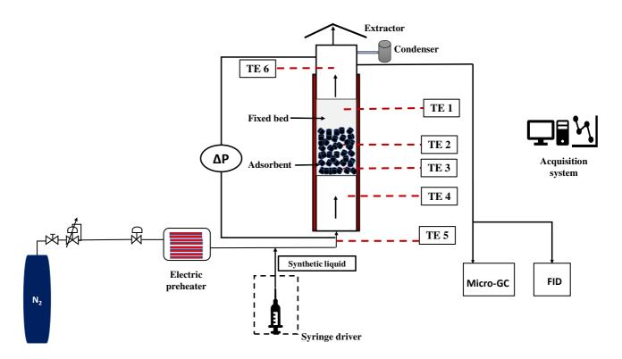
Fig. 1. Representative diagram of the post-pyrolysis reactor.
