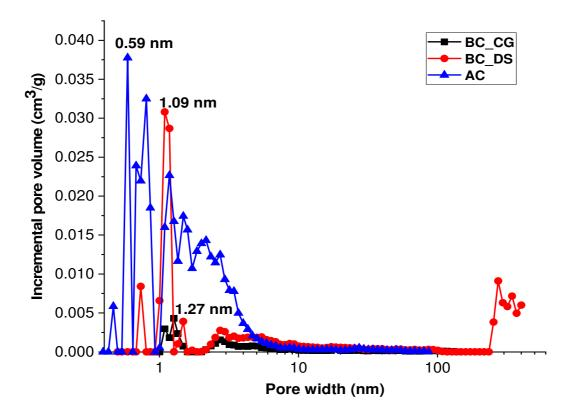
Fig. 2. Pore size distribution of BC\_CG, BC\_DS, and AC.
