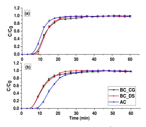
Fig. 3. Breakthrough curves of thiophene at 500 °C; 0.20 Nm<sup>3</sup>/h; (a) synthetic mixture 1; (b) synthetic mixture 2.
