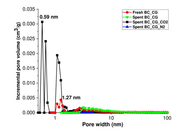
Fig. 7. Pore size distribution of Fresh BC\_CG , Spent BC\_CG , Spent BC\_CG\_CO<sub>2</sub>, and Spent BC\_CG\_N<sub>2</sub>.
