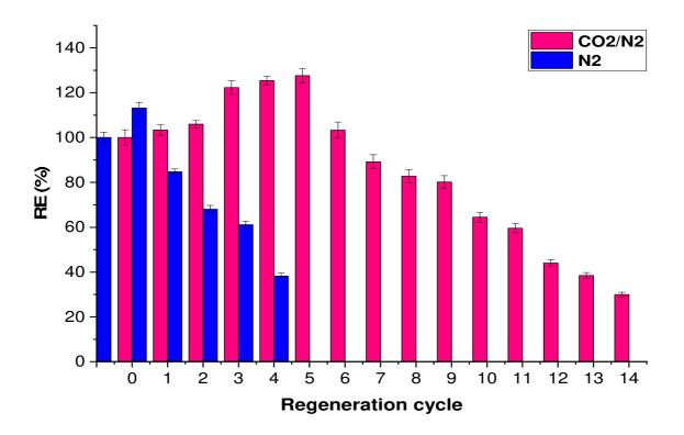
Fig. 6. Evolution of the regeneration rate according to the regeneration cycle/method. According to the literature, thermal regeneration is the most widely used regeneration method and one of the most economical and efficient methods. On the other hand, several references have also applied regeneration by gasification using either steam or CO<sub>2</sub>. The comparison of
