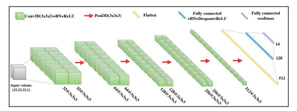
Figure 3: Architecture of our 3D CNN.
