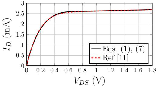
Fig. 1. DC characteristics  $I_D \times V_{DS}$  with  $V_{GB} = 1.8$  V of the n-channel MOSFET with  $W/L = 5 \mu\text{m}/0.18 \mu\text{m}$  from the  $0.18 \mu\text{m}$  CMOS technology using equations (1), (7) and [11].
