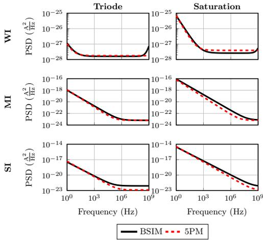
Fig. 7. Noise simulation results of the power spectral density (PSD) for SVT n-channel transistor with  $W/L = 5 \mu\text{m}/0.18 \mu\text{m}$  from  $0.18 \mu\text{m}$  CMOS process. Operating points: in triode  $V_D = 13 \text{ mV}$  and saturation  $V_D = 1.8 \text{ V}$ ; in weak inversion (WI)  $V_G = 100 \text{ mV}$ , moderate inversion (MI)  $V_G = V_{T0} = 528 \text{ mV}$ , strong inversion (SI)  $V_G = 1 \text{ V}$ .
