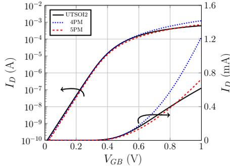
Fig. 4. DC characteristics  $I_D \times V_{GB}$  with  $V_{DS} = 500 \text{ mV}$  of the LVT n-channel MOSFET with  $W/L = 1 \mu\text{m}/60 \text{ nm}$  from a 28-nm FD-SOI technology.
