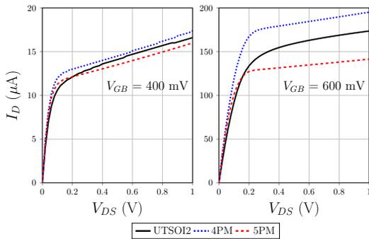
Fig. 5. DC characteristics  $I_D \times V_{DS}$  with  $V_{GB} = 400 \text{ mV}$  and of  $V_{GB} = 600 \text{ mV}$  of the LVT n-channel MOSFET with  $W/L = 1 \mu\text{m}/60 \text{ nm}$  from the 28-nm FD-SOI technology.
