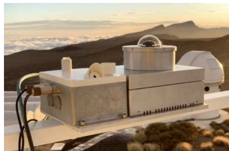
Figure 3: Miratlas Integrated Sky Monitor.
