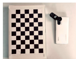
Fig. 2. Complete setup for shading estimation: a calibration pattern on the left, a smartphone with clipped-on fisheye on the right.
