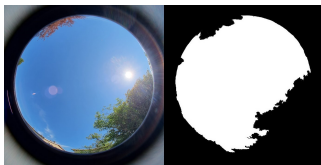
Fig. 4. Sky image above our solar panel test setup. Original version on the left, converted to white and black to distinguish sky and obstructions respectively on the right.
