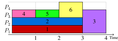
(d) Scheduling made with the same jobs but with a different utilization profile, WRT = 37 (different), HC = 23.5 (different).
