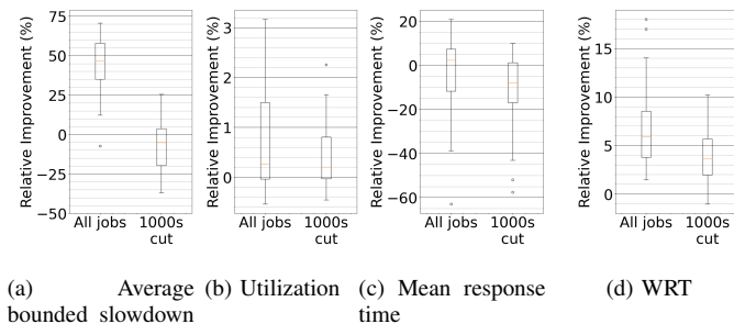
Fig. 6: Evolution of the Relative Improvement of EXACT over USER-WALLTIME with several metrics when deleting the jobs that last less than 1000s (Theta data). y-axis are not the same.
